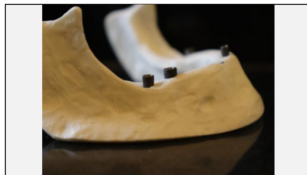
Figure 1. Styrofoam Model with Embedded Implants with 4-5 Threads Exposure
