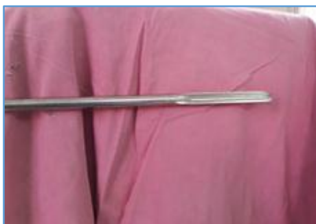
Figure 1. Modified Innovative Reamer (with long straight flutes)
