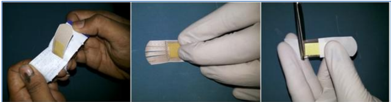
Fig. 1: Steps in Preparing Strips from Band-Aid
