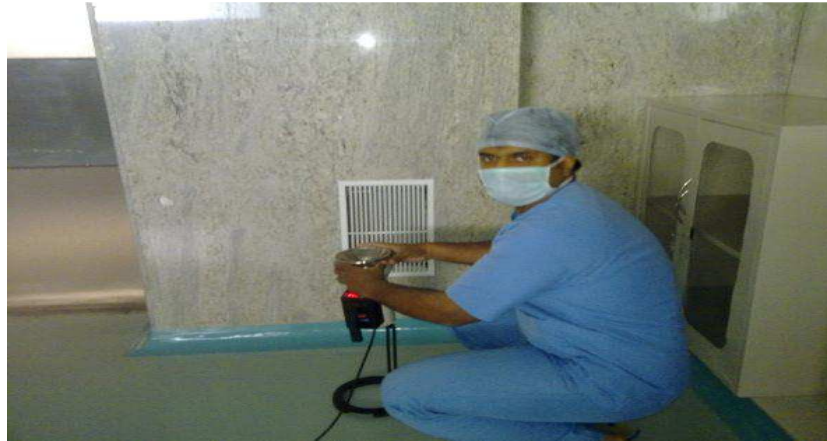
Pictures – 6 . Air sampling using the device.
