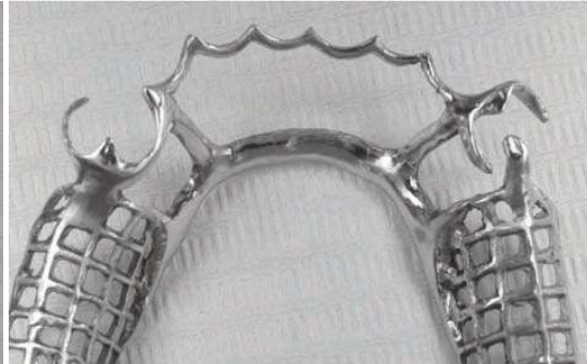
b. Repaired with laser welding
