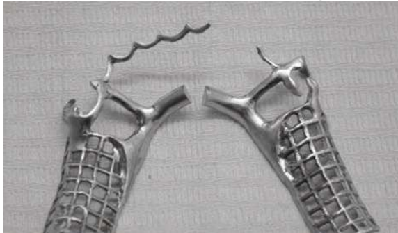
a. Cracked continuous bar & lingual bar.
