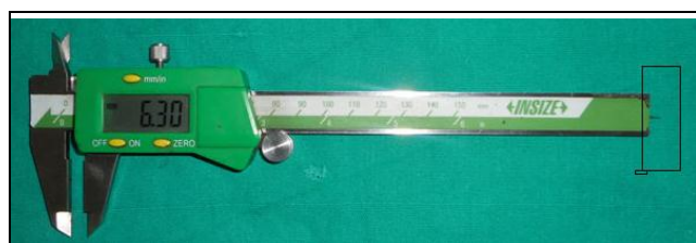
Figure 2. Modified Digital Vernier Calliper used for Assessing Gingival Thickness
