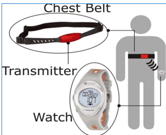
Figure 3. Mechanism of Working of Polar HR Monitor
